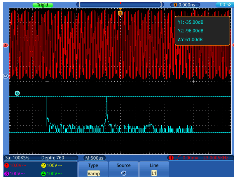
Figure 0-12 Wave of Vamp cursor measurement
