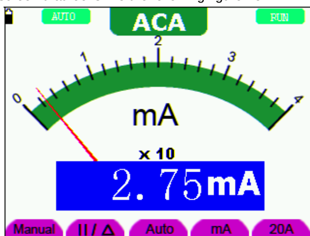
Figure 25: AC Current Measurement for 400 mA
