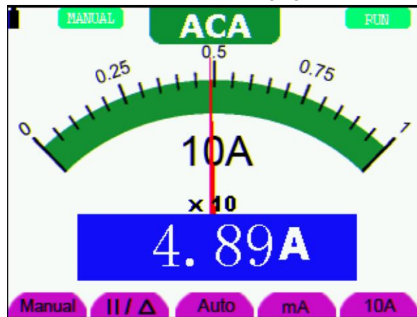
Figure 26: AC Current Measurement for 10A
