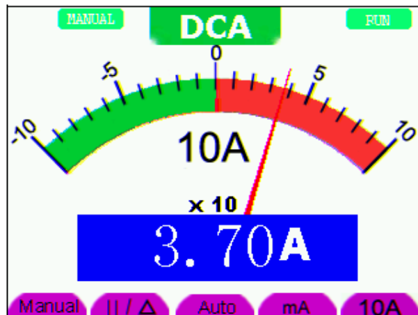
Figure 24: DC Current Measurement for 10A
